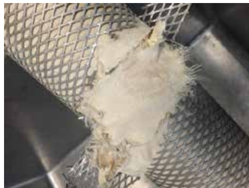
Figure 8. Sterile process of destructive disassembly a Donaldson sterile air filter, model P-SRF N 30/30 (0.2 \mu\text{m} absolute, expanded PTFE filter membrane) for bacteriophage diagnostic testing. Note the dark water staining on protective prefilter barrier layer on the filter.
