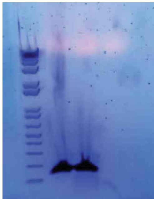
Figure 5. DTL-phage amplicons generated from PCR (DTL-phage 40 set, Table 1 ) and separated by 1% agarose gel electrophoresis. Lane 2 is a positive control of purified DTL-phage DNA, lane 3 is a seed fermenter sample containing 2 \times 10^4 particles of DTL-phage per mL, and lane 4 is a sterile water negative control. Lane 1: Invitrogen E-Gel 1 Kb Plus Express DNA Ladder (part #10488091) 100–5000 bp.
