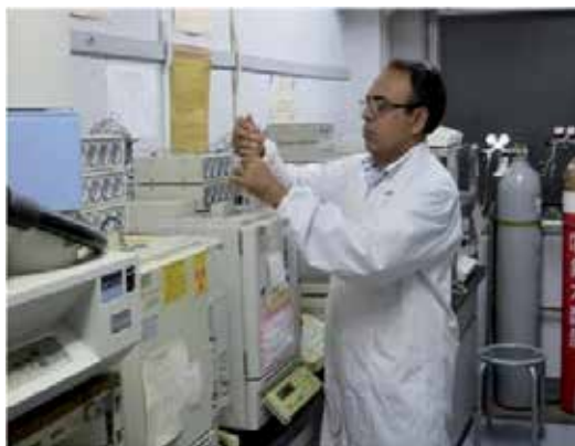
Figure 4. Injecting air samples into GC for determination of CH 4 and N 2 O concentrations.
