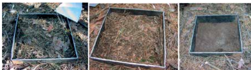
Figure 2. Sampling of forest floor under Scots pine stands—horizons L—litter (left), F—fermentation (in the middle) and H—humus (right).
