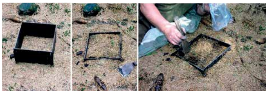
Figure 1. Sampling of forest floor L layer using steel frames (25 × 25 cm) in Norway spruce stands.
