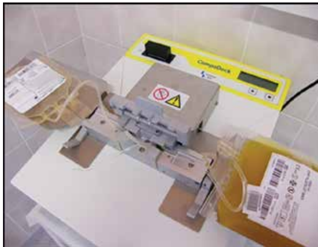
Figure 2. Sterile connection of the container with PLTs contained DMSO to container for freeze.
