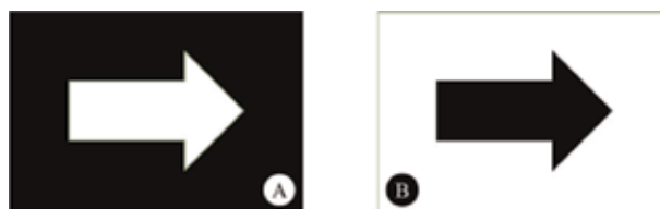
Figure 4. Different forms of mask used in photolithography. (A) The mask intend for positive substrate photoresist and (B) the mask for negative photoresist.
