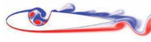
Figure 12. The vorticity contour plot over the airfoil with a cavity [63].
