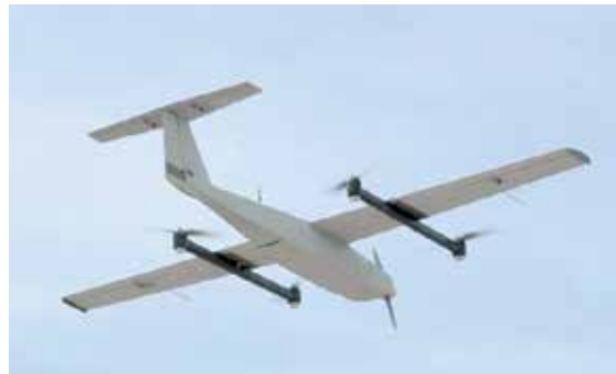
Figure 4. A hybrid fixed-wing-multi-rotor UAV [9].
