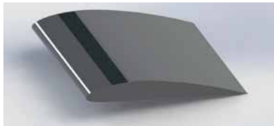
Figure 15. Representation sketch of the roughened airfoil.
