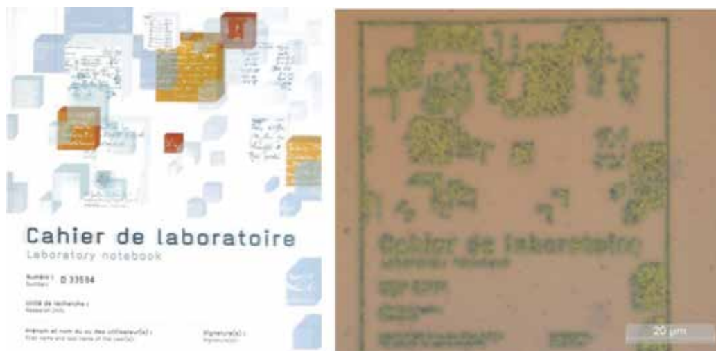
Figure 13. The color printed image fabricated by the DLW method on Au film. Left: a real "experiment book". Right: a plasmonic image of corresponding book at microscale.
