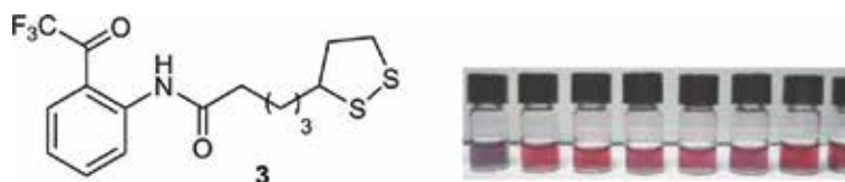
Figure 13. (Left) Ligand used to cap gold nanoparticles for detection of fumarate. (Right) Color changes of an aqueous solution of AuNPs capped with 3 upon addition of various analytes (as sodium salt). From the left: fumarate, maleate, oxalate, malonate, succinate, glutarate, propionate, and 4-pentenoic acid.
