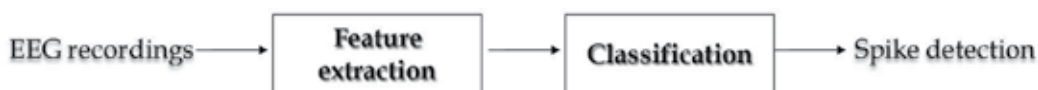
Fig. 2. The spike detection problem seems to be broken down into two main stages: feature extraction and classification. This can be viewed as mapping the N -dimensional EEG pattern space to a F -dimensional feature space (where N \geq F ) and then performing classification in the feature space. In the case of use of raw EEG recordings without feature extraction, this can be seen as the case where the N -dimensional EEG space is mapped onto an identical N -dimensional feature space where classification then takes place (James, 1997).
