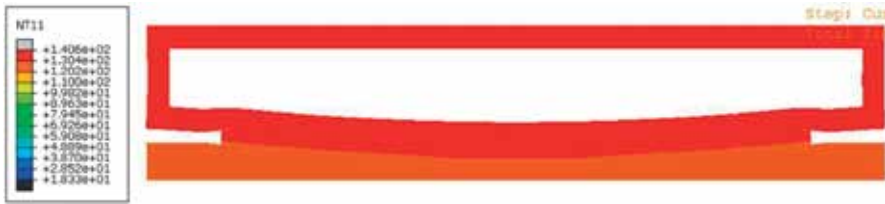
Figure 16. Nodal temperature results at t = 274 s (relative to current load step).
