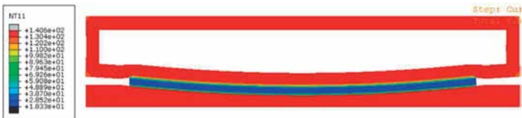
Figure 13. Nodal temperature results at t = 120 s (relative to current load step).
