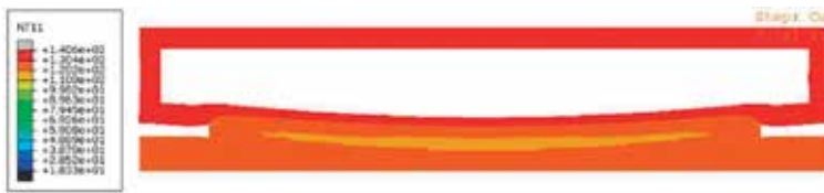
Figure 15. Nodal temperature results at t = 147 s (relative to current load step).
