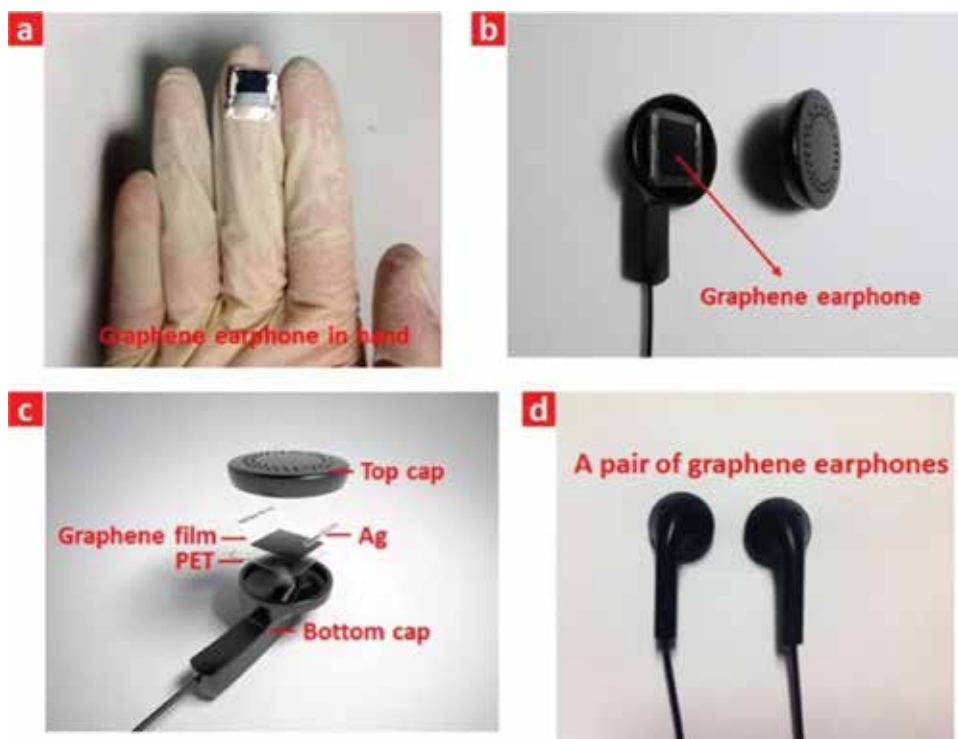
Figure 12. The demonstration of graphene earphone [13]. (a) Graphene earphone in hand. (b) View of the graphene earphone in a commercial earphone casing. (c) Exploded view of a packaged graphene earphone. (d) A pair of graphene earphones in its final packaged form.
