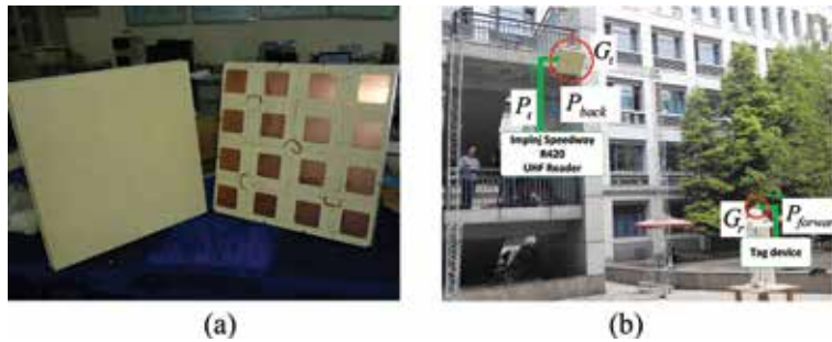
Figure 9. (a) 4 x 4 CP microstrip patch antenna array fabricated prototype and (b) experimental setup for the ETC antenna array system measurement.
