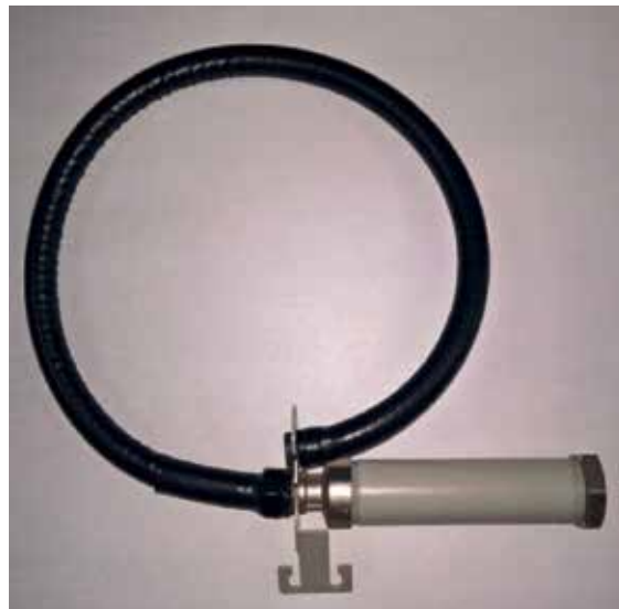
Figure 15. Photo of the device for registration of current derivative from the source of powerful EMI action in the near field based on the 4th generation lightning current recorder.
