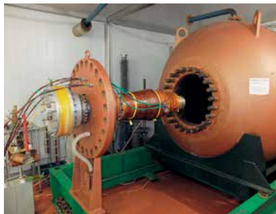
Figure 11. EMG assembly, before installation in the explosion protection chamber.
