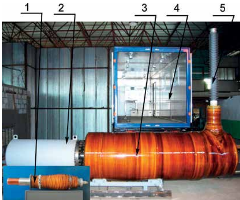
Figure 2. The main elements of the lightning current generator: 1—EMG; 2—explosion protection chamber; 3—pulse transformer; 4—container body; 5—bushing insulator.
