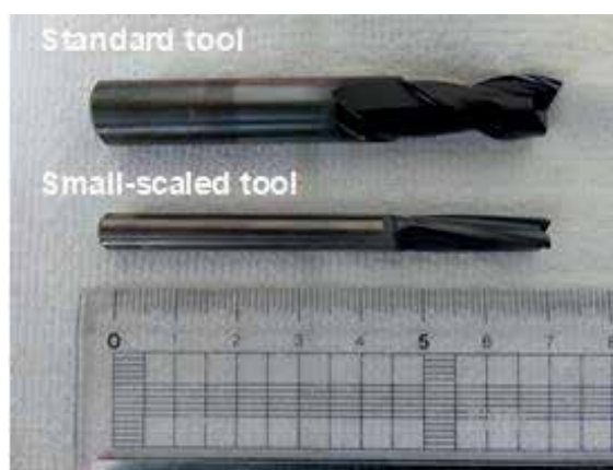
Figure 8. Two diamond-coated end-milling tools as a specimen for plasma ashing process.
