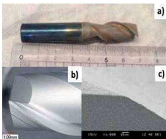
Figure 11. Ashing of CVD-diamond coating on the WC (Co) standard specimen under (250 V; -500 V; 45 Pa; 3.6 ks). (a) Surface of ashed specimen before cleansing, (b) Ashed tool edge, (c) SEM image of tool edge.
