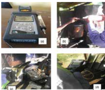
Figure 4. (a) KANE AUTOplus gas analyzer, (b) blended fuel being poured into the fuel tank of diesel engine, (c) gas emission analysis and (d) saving of analysis results on analyzer.
