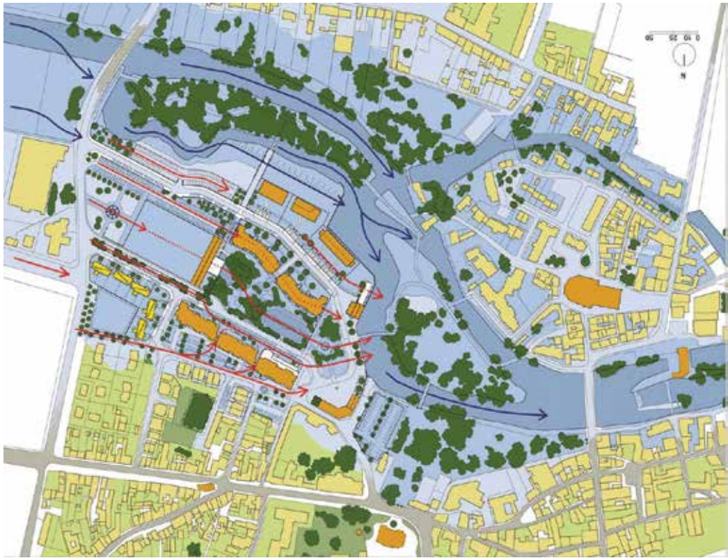
Figure 5. Romorantin, a study of hydraulic transparency during a 100-year flood in “Matra” district (the flow of water through the district marked in red). Source EDL - Eric Daniel Lacombe.
