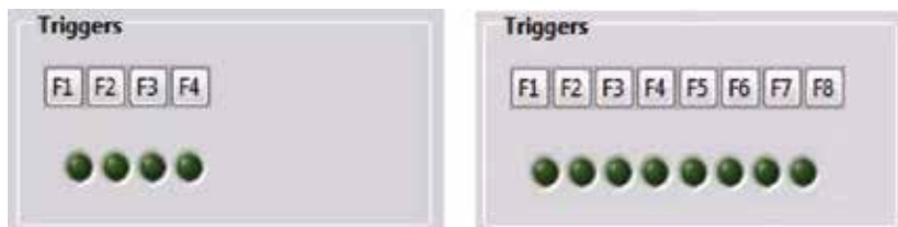
Figure 9. (Courtesy of NIRx Medical Technologies) shows different trigger signals that can be used to set the end and the beginning of psycho-physiological stimuli; the marker is set by clicking on the respective button (e.g., F1) or by pushing F1 key on the computer keyboard.
