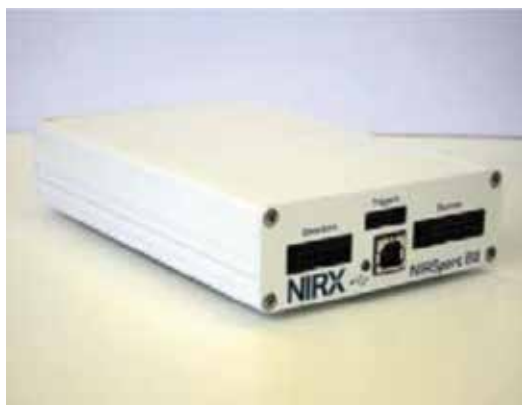
Figure 2. (Courtesy of NIRx Medical Technologies) NIRSport 8 \times 8 imaging system; detectors and sources must be placed in the corresponding slot, equally for triggers sent to the software through a specific equipment (if necessary), the connection USB cable and, on the other side, the power supply connector.
