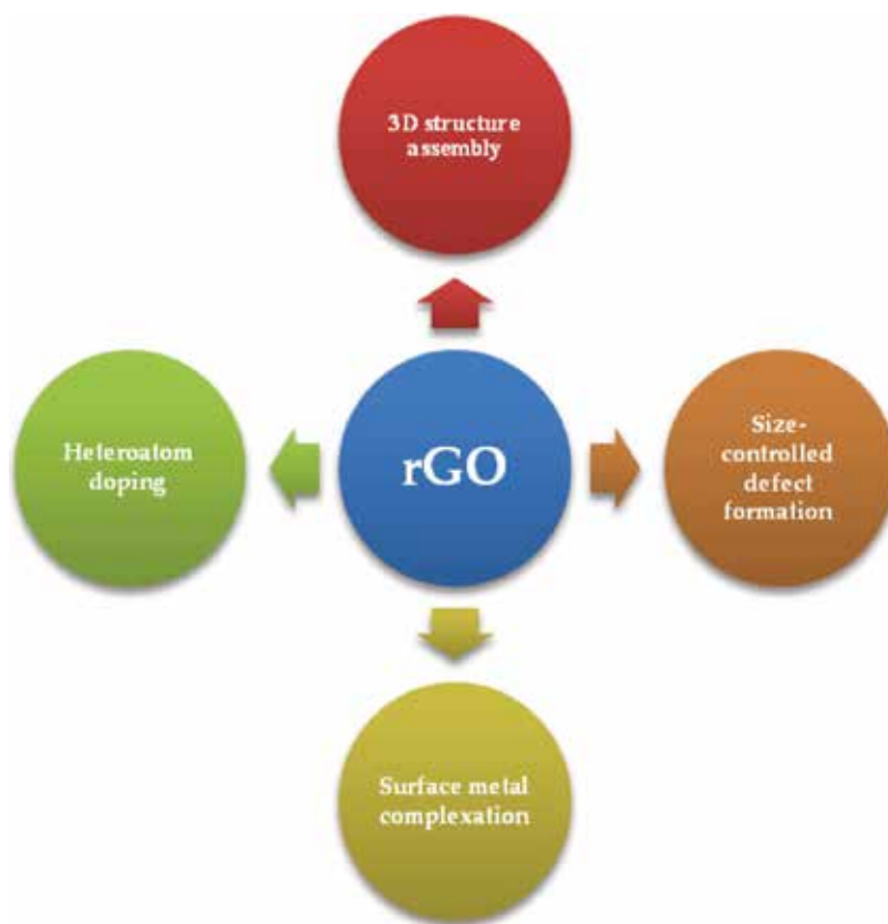
Figure 1. General schematic roadmap of defect engineering strategies in reduced graphene oxide support materials for achieving advanced energy conversion.
