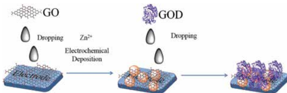
Figure 5. The preparation scheme of ZnO/GO/GOD-based glucose biosensor [11].
