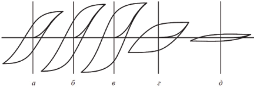
Figure 22. Preisach model: effect of increasing the parameter a_1 on the form of hysteresis loops.
