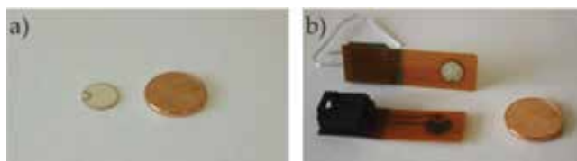
Figure 1. Types of transducers, (a) single transducer with wrap-around electrode from PICeramic, (b) embedded transducer, Accellent SMART layer ® .
