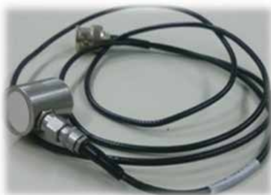
Figure 3. A typical AE sensor with connecting cable.
