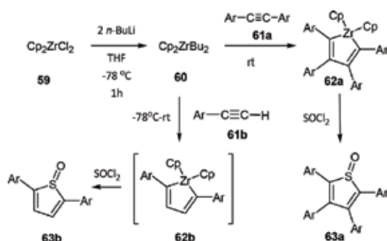
Scheme 15. Synthesis of tetraarylthiophene S -oxides 63a/b by reaction of tetraarylzirconacyclopentadienes 62a/b with SOCl_2 .
