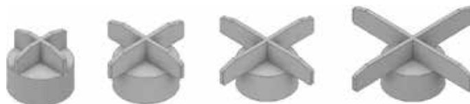
Figure 2. Magnetic impeller with increasing blade diameter.
