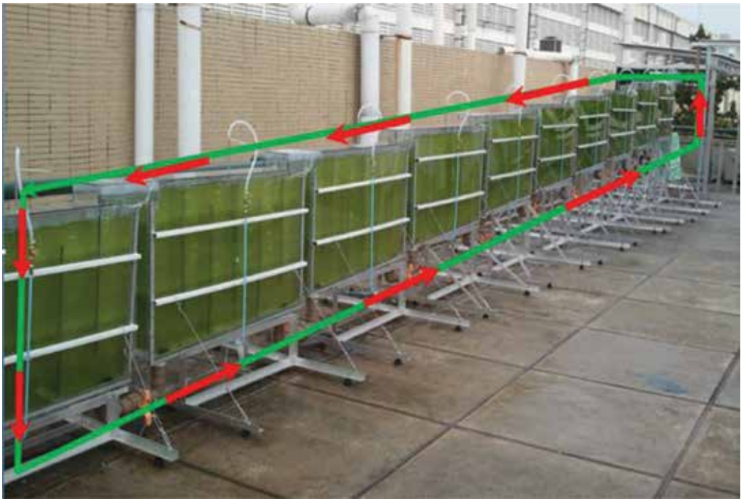
Figure 6. Recirculation of cultivation system along the ten photobioreactors at GreenTech.
