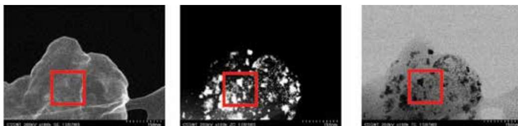
Figure 3. Co-localized SE—secondary electrons (left), ZC—phase contrast (middle) and TE—transmission electrons (right) images of the Pt/rGO x sample.
