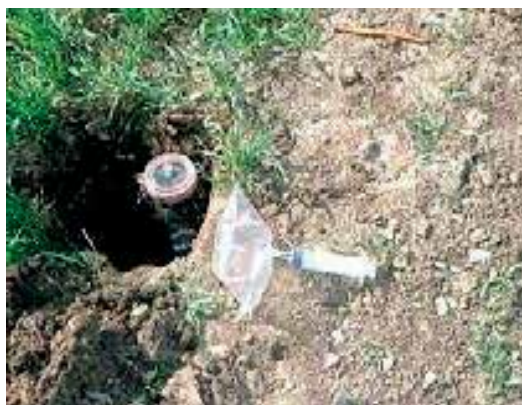
Figure 4. Incubation pot before it was buried and bag and syringe with acetylene.
