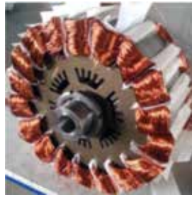
Figure 12. Stator windings of OR-SRM at manufacturing stage.
