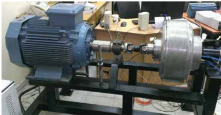
Figure 14. OR-SRM test bed.
