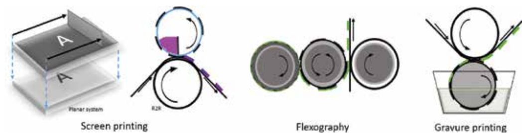
Figure 2. Schematic of contact printing techniques.
