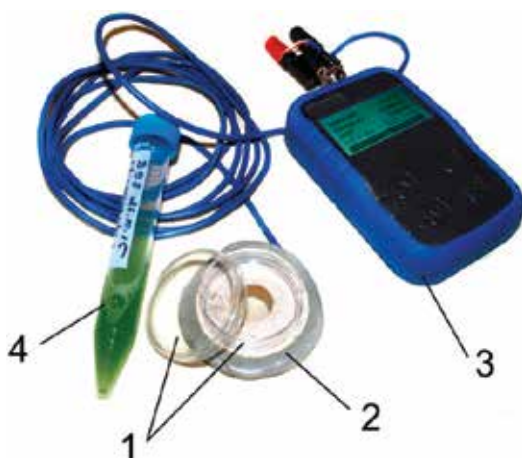
Figure 5. The developed device for laboratory ultrasonic treatment of cyanobacterial culture. (1) Plastic petri dish, (2) ultrasonic emitter, (3) generator of ultrasonic frequencies and (4) sample culture.
