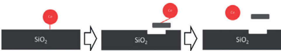
Figure 10. The schematic mechanism of oxide removal rate by ceria abrasive.
