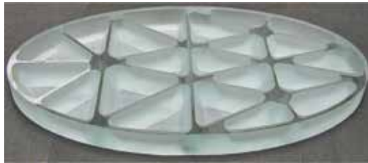
Figure 16. 250 mm (major axis) elliptical mirror with pockets milled to 9.5 mm deep.
