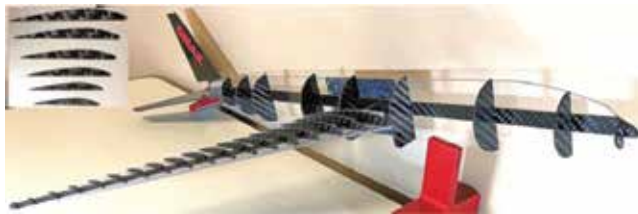
Figure 10. A Boeing 777 aircraft model assembled from AWJ-cut components made from carbon fiber [3].
