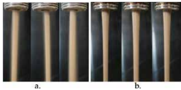
Figure 4. Flow patterns of unprocessed and processed 320-mesh garnet [7] (a) Unprocessed (b) Processed.
