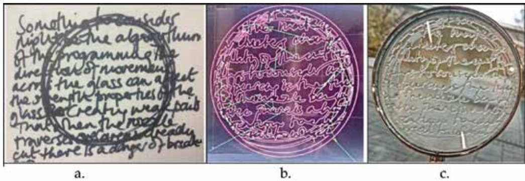
Figure 22. Processes for AWJ-machining of handwriting on glass [15] (a) Initial drawing sketch (b) Tool paths and (c) Micro glass handwriting.
