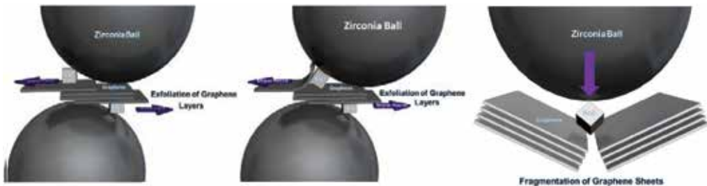
Figure 5. Exfoliation and fragmentation of graphene. Source: Ref. [1], Copyright @ 2017 Word Scientific.
