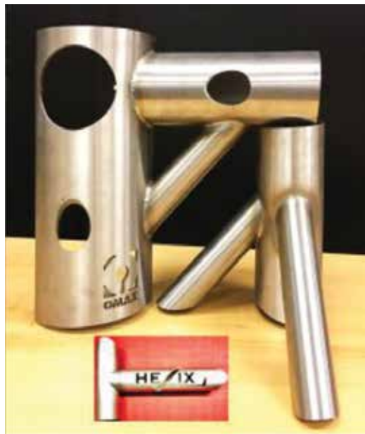
Figure 14. AWJ-cut “Fish mouth” weld joints.
