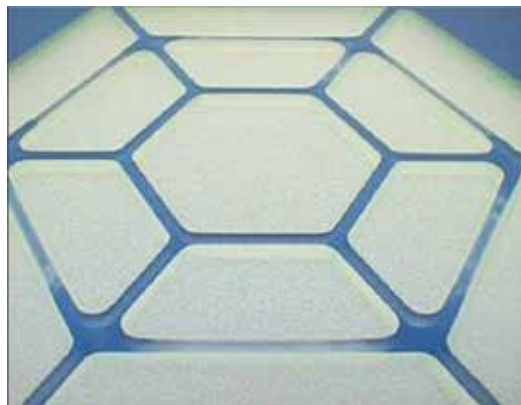
Figure 19. Superimposing successive milling passes to generate flat surfaces.
