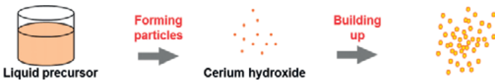
Figure 13. Synthesis of nano-sized cerium hydroxide abrasive (reprinted from Ref. [33] with permission from authors).
