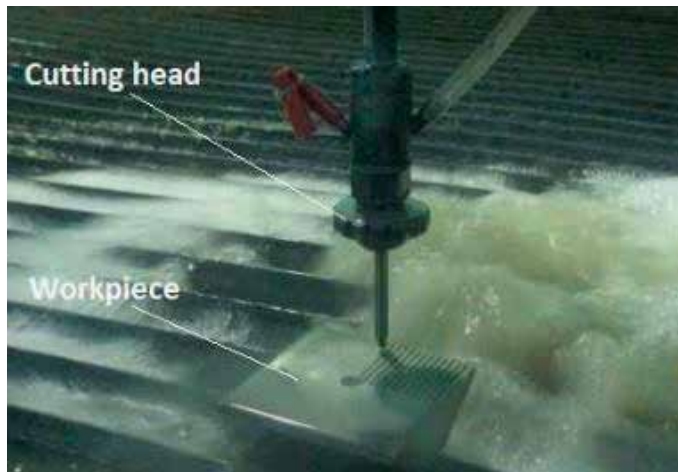
Figure 4. Experimental setup for determination of maximum depth of cut.
