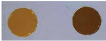
Figure 4. Photographs of pristine reference Kapton (left) and a radiation damaged Kapton sample (right) taken after an electron dose of 5.6 \times 10^7 Gy. Right picture was taken after 2 min of air exposure.
