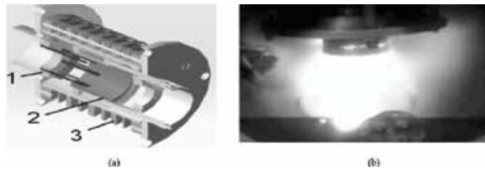
Figure 9. (a) Experimental sample: 1- cathode, 2- anode, and 3- permanent magnets system; (b) plasma jet in high-current operation mode.
