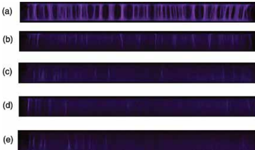
Figure 2. Discharges at different airflow speeds. (a) Flow speed v = 0 m/s, (b) v = 10 m/s, (c) v = 35 m/s, (d) v = 50 m/s, and (e) v = 100 m/s. Exposure time is 1/1250 s.
