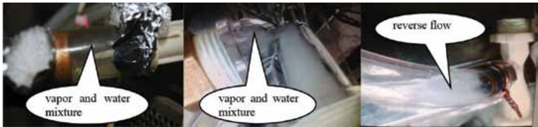
Figure 7. The flow state of the water vapor in the ejector.
