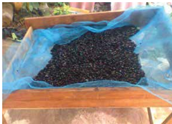
Figure 5. Draining of OPKSC after imbibition to obtain saturated surface dry (SSD) status.
