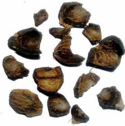
Figure 3. Different size of Oil Palm Kernel Shell for the concrete mixing.
