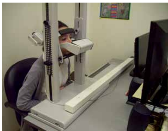
Fig. 2. Mobile Eyebrain Tracker (Mobile EBT®) used to record eye movements from both eyes in children.
