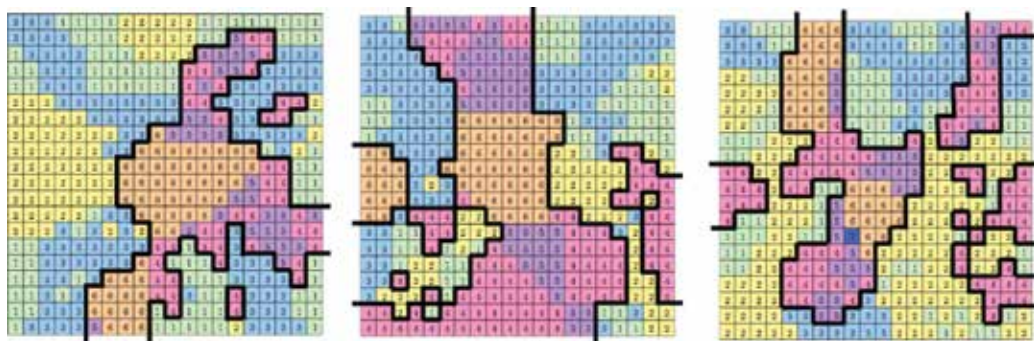
Figure 9. Category maps of Subjects A–C. The grids correspond to the units on the mapping layer of CPNs. Labels 1–7 denote face-up sleeping, right sleeping left sleeping, longitudinal sitting, lateral sitting, terminal sitting, and left the bed.
