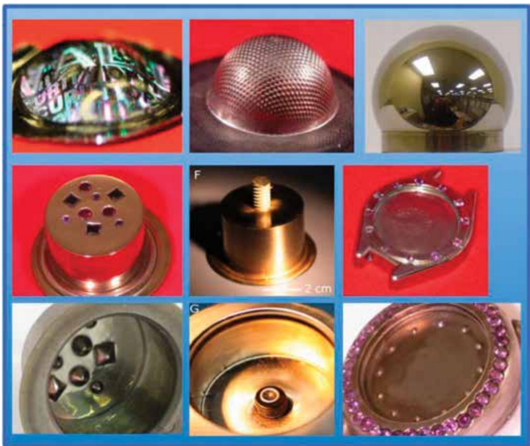
Figure 3. These shapes were previously unachievable with any other metal processing method that can be fabricated by blow molding [46].
