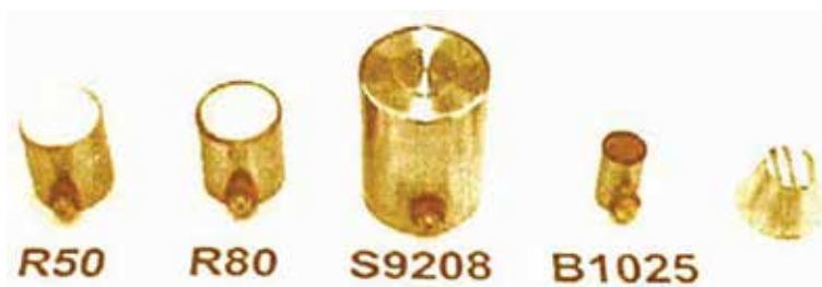
Figure 5.1 Acoustic emission transducers for AE signals from high-power microwave tubes. The rightmost object is aluminum matching buffer piece.
