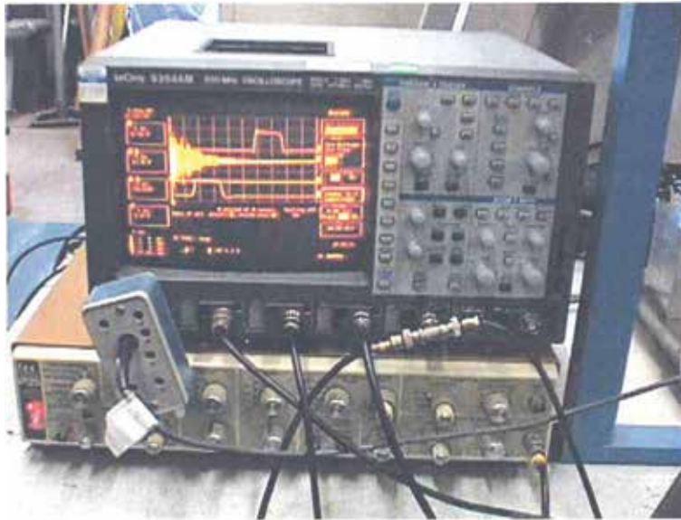
Figure 6.3. AE signal from magnetron on LeCroy digital oscilloscope.
