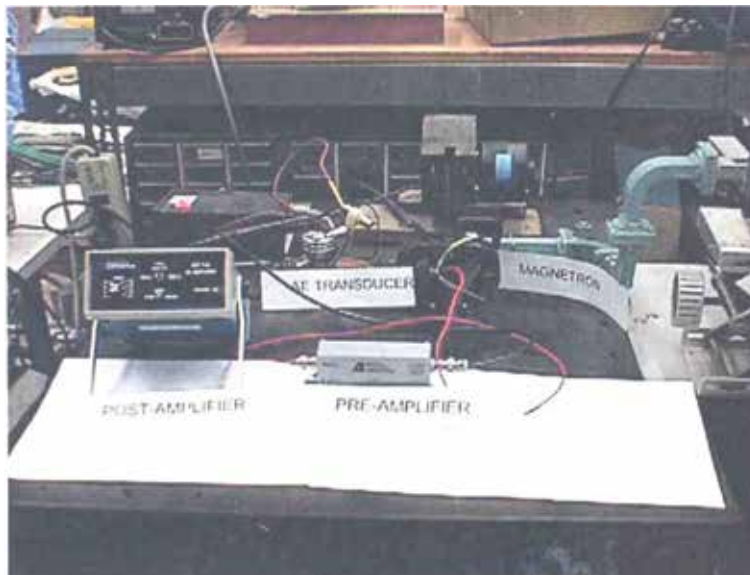
Figure 6.2. Photo of setup of AE equipment next to magnetron.
