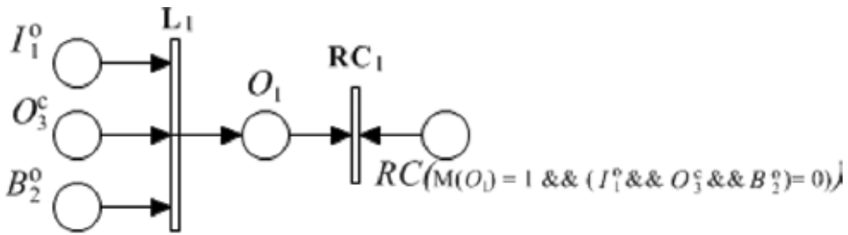
Figure 11. PN model of logic AND.
