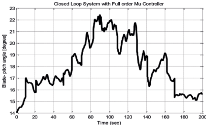
Figure 13. Pitch angle adjustment using the \mu controller.
