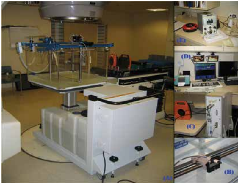
Figure 2. Varian linear accelerator for clinical use, and the basic equipment for radiotherapy calibrations. (A) Computerized water phantom system, (B) PTW ionization chamber N31003 no. 975; (C) Scanditronix Wellhofer; (D) Fixed computer system; and (E) Keithly CNMC electrometer. Courtesy of Dr. Carlos Esquivel, from Cancer Therapy & Research Center, San Antonio, Texas, USA.
