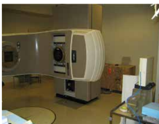
Figure 6. Experimental set-up for TBI calibration with a linear accelerator at the treatment distance (3.50 m), and an ionization chamber installed inside the PMMA solid phantom. Calibration process conducted at the Cancer Therapy & Research Center, San Antonio, Texas, USA. Courtesy of Dr. Carlos Esquivel, from Cancer Therapy & Research Center, San Antonio, Texas, USA.
