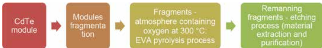
Figure 6. Summary of ANTEC solar GmbH recycling process for CdTe modules [43].
