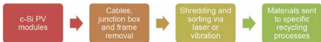
Figure 4. Summary of PV cycle recycling process for c-Si modules [25].
