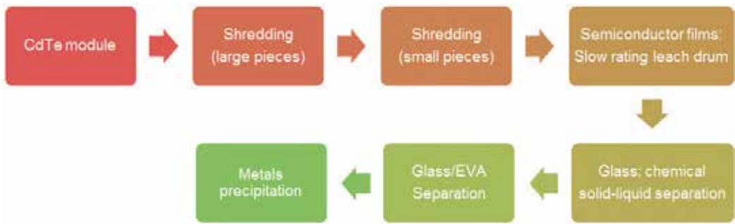
Figure 5. Summary of first solar recycling process for CdTe modules [21].
