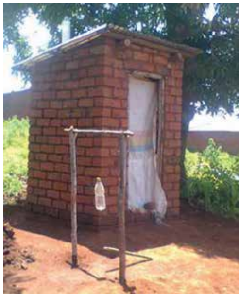
Figure 1. Tippy tap close to toilet for hand washing in rural areas of Malawi.
