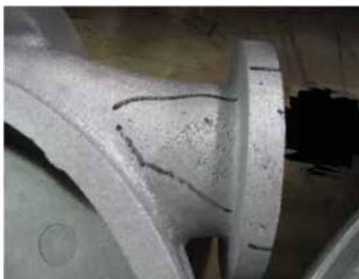
Figure 2. Pump body casting of Al-Si alloy with visible blow-holes on the surface, produced in the sand mould - hand moulding technology.
