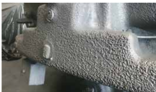
Figure 4. High-dimensional iron casting with visible gaseous defects on the surface, produced in the sand mould-hand moulding technology with the application of moulding sand with furan resin.
