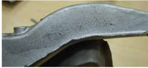
Figure 5. Casting of Al-Si alloy with visible blow-holes on the surface, produced in the metal mould-low-pressure casting technology.
