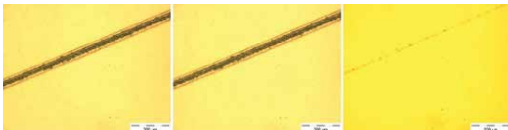
Figure 7. Scratch recovery for 2Ph2Epo65, 10 × magnification. From left to right: at room temperature, at 120°C, after additional annealing for 30 min at 120°C.
