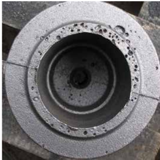
Figure 1. Iron casting with visible blow-holes on the surface, produced in the mould of wet bentonite moulding sand high-pressure technology.
