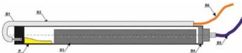
Figure 7. Structure of the measuring sensor (B) for the thermal volumetric investigations [12].
