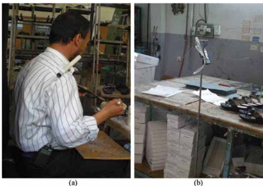
Figure 1. Atmospheric metrology in a semi-industrial shoe manufacturing company. (a) Individual sampling at the “uppers preparation workstation and (b) ambient sampling at the “finishing workstation.
