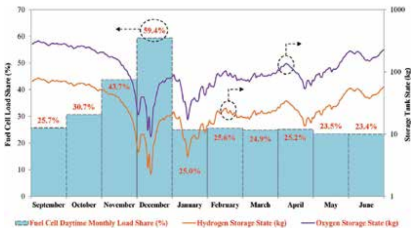
Figure 8. State of energy storage tanks and fuel cell share on monthly basis [19].
