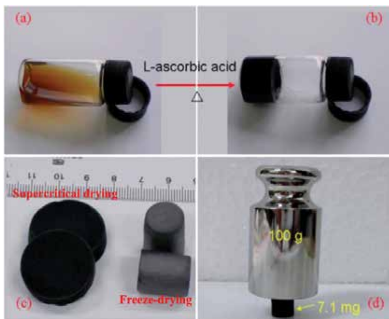
Figure 1. Digital photos of the aqueous suspension of graphene oxide (a), the graphene hydrogel in a vial (b), the graphene aerogels obtained by supercritical \text{CO}_2 drying and freeze-drying (c), and a graphene aerogel supporting a counterpoise (d) [17].
