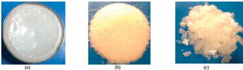
Figure 2. Phase-change materials in their original states, (a) paraffin wax, (b) stearic acid, (c) sodium hydroxide.
