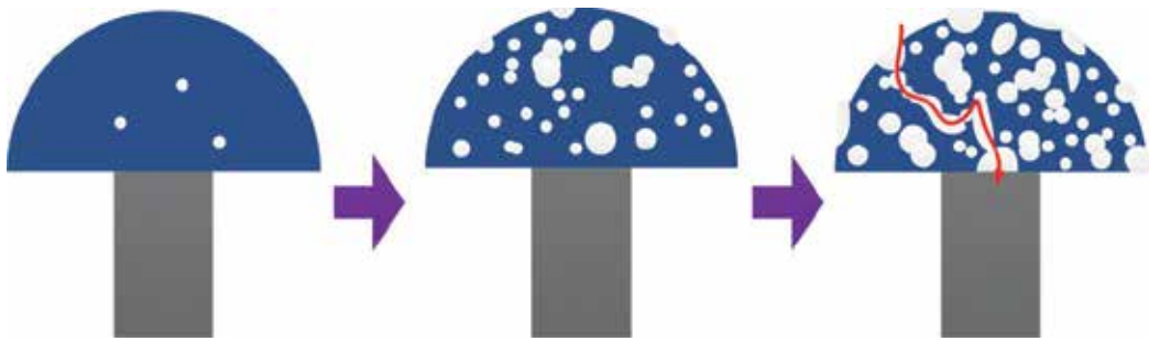
Figure 12. Nucleation, growth and saturation stage diagram of PCM cell in the SET process.
