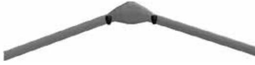
Figure 3. A schematic 3D view of a very flexible high-aspect-ratio wing.
