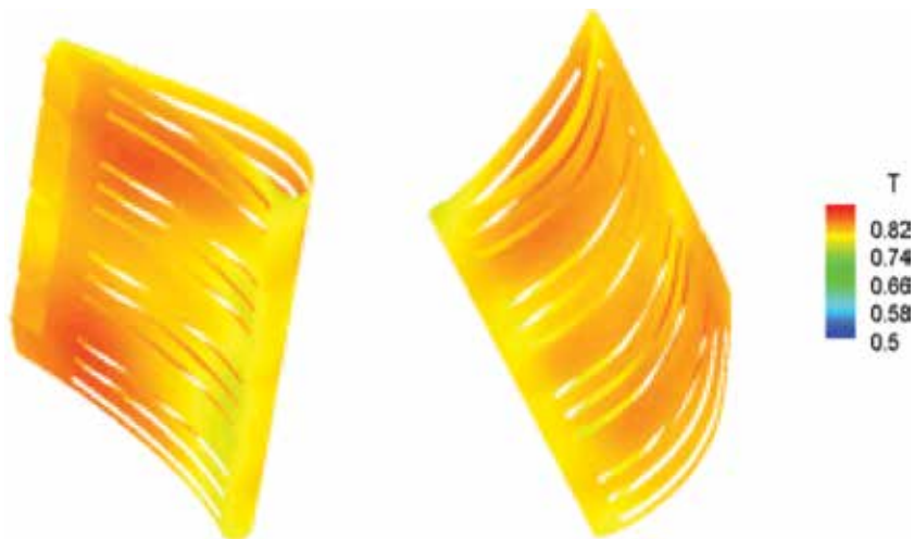
Figure 7. Temperature contours at the internal surfaces of the pressure and suction sides.
