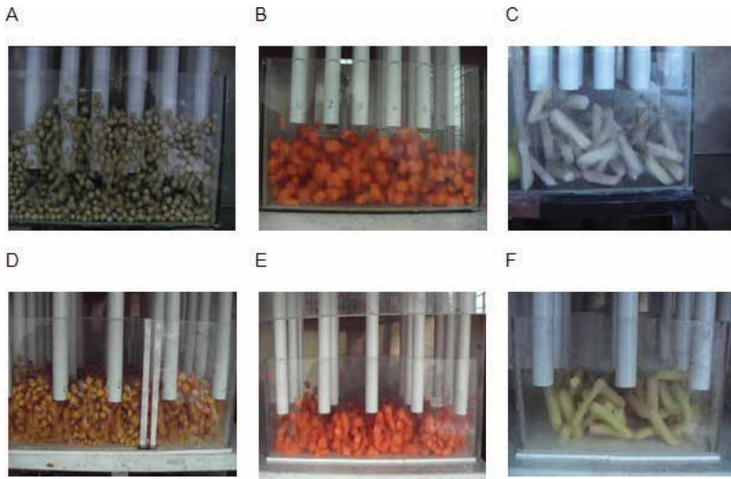
Figure 5. The view of impingement fluidization of different products [33].
