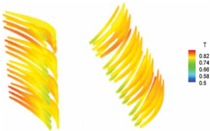
Figure 8. Temperature contours at the cooling fin surfaces.
