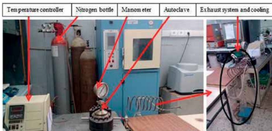
Figure 7. PARR autoclave-type pressure reactor and solvent removal system.
