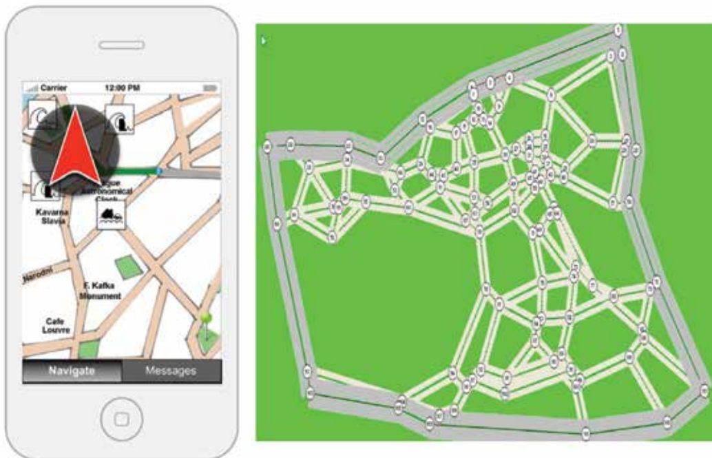
Figure 4. Navigation on the flooding app and the graph representing the street network of the city.
