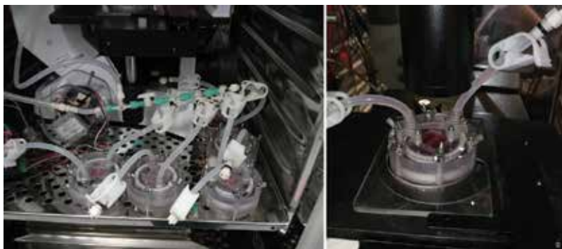
Figure 4. Cultivation chambers used for mechanical stimulation (left). The use of transparent surfaces allows microscopic live-cell imaging (right).
