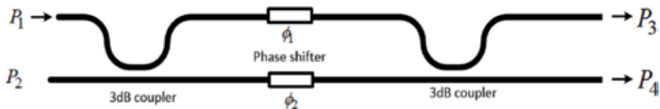
Figure 3. MZI cell based on directional coupler type II.
